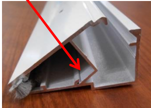
Engage lip into groove
